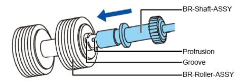
(2) Fit the left end of the BR-Shaft-ASSY in the slot (①), then install the rest of the shaft in place (②).
