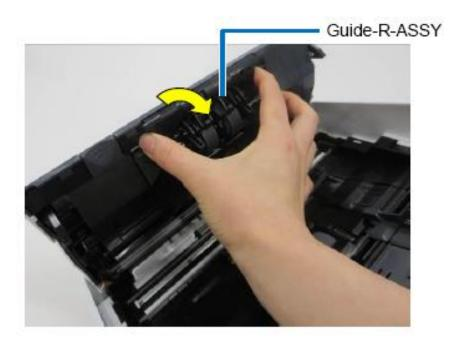
(3) Lift the BR-Roller-ASSY on the right side, remove the right-side shaft (1), and pull out the left-side shaft from the slot (2).
