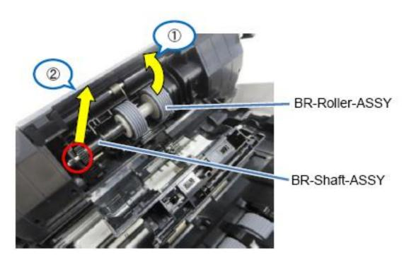
(4) Remove the BR-Roller-ASSY from the BR-Shaft-ASSY.
